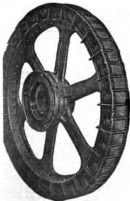
FIG. 7,787.—Rotor field of General Electric 360 horse power self-starting type synchronous motor, showing the amortisseur or squirrel cage starting winding in the pole faces. The synchronous motor can use a high resistance squirrel cage
