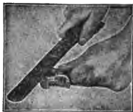
FIG. 6,343.— Battery repairs 43. Using an ordinary pocket knife, clean the inside of the connectors, removing all dirt and oxides. Clean the tops of the connectors with a rasp file to remove dirt and oxide.
