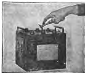
FIG. 6,341.— Battery repairs 41. After the form is removed there is always an excess of sealing compound. This can be scraped off with a hot putty knife.
