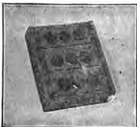
FIG. 6,339.— Battery repairs 39. Wooden form used for properly holding the covers down while the compound is cooling.
