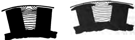
FIGS. 7.707 and 7.708.—Diagram showing respectively the character of stray field between adjacent straight poles, and between adjacent poles with shoes.
