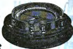
FIG. 6,683.—Breguet upright galvanometer with glass shade.
