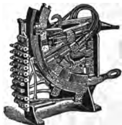
Figs. 8,108 to 8,115.—Controller of the Rauch and Lang electric vehicles. It is of the flat radial type. Two movable copper leaf contacts of ample size make all commutations necessary to obtain the various speeds. Five speeds forward and reverse are provided.
