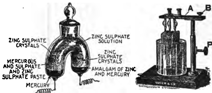
FIG. 6,830.—Clark cell, or standard for the International volt . The pressure is 1.434 volts at 15° C., decreasing .00115 volt for each increase of 1° C.
