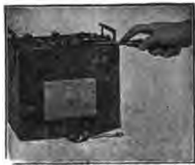
FIG. 6,307.— Battery repairs 7. Using a heated screw driver, chisel or a plumber's lead scraper dig out the compound around the edges of the covers.
