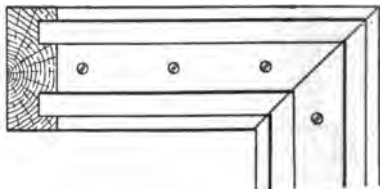
FIGS. 6,973 and 6,974.—Cutting mitered corners of wooden moulding. All standard moulding is 1\frac{1}{2} ins. wide. Hence, measure 1\frac{1}{2} ins. from end obtaining point L, and cut on line drawn from L to F. Similarly cut other pieces and they will go together as in fig. 6,974. A miter box will save much time and is more accurate.
