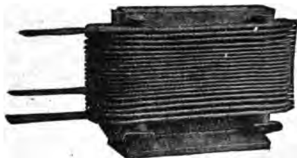
FIG. 6,599.—Commutating pole of Westinghouse commutating pole rotary converter. The commutating poles are similar in general construction to the main poles. The coils are of bare copper strap wound on edge. Ventilating spaces are provided between the pole and coil and between turns. The copper winding is bare except for a few turns at each end. Insulating bolts retain the turns in their proper position.
