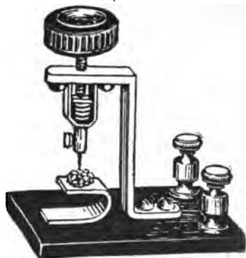
FIG. 8,486.—Mascot rotary variable condenser, the knurled hand rubber knob has an arrow head pointer to register on a celluloid scale.
