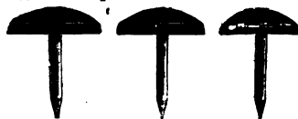
FIGS. 8,350 to 8,353.—Milonite nails and method of tacking two insulated wires. The nails are colored to match insulation and the wires can be tacked down without cutting or injuring the insulation.
