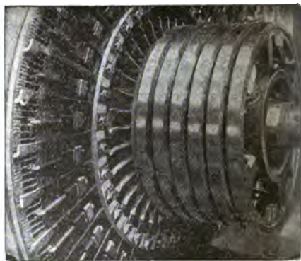
FIG. 6,583. —General Electric converter collector ring brush rigging. The brush and brush holders used on the collector rings illustrate changes in modern synchronous converter practice. The brushes are made of combined copper and graphite by a new process and have the appearance of solid copper.
