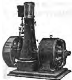
FIG. 7,895.—Triumph dynamo set with upright slide valve engine.
