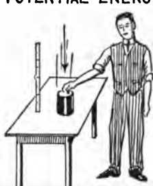
FIGS. 6,466 to 6,468.—Mechanical analogy of wattless current. If a man lift a weight any distance as from the position of fig. 6,466 to position of fig. 6,467, he does a certain amount of work on the weight giving it potential energy. When he lowers it to its original position, as in fig. 6,468, the weight loses the potential energy previously acquired, that is, it is given back to the man, the "system" (man and weight) having returned to its original condition as in fig. 6,466. During such a cycle, the work done by the man on the weight is equal to the work done by the weight on the man and no useful external work has been accomplished.
