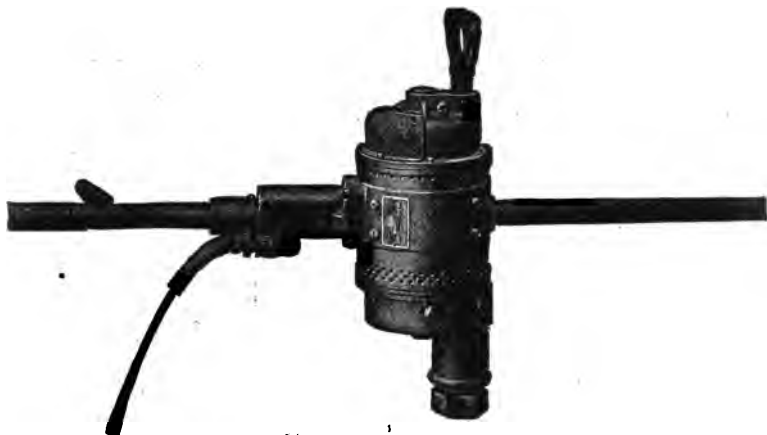
FIG. 7,927.—Chicago "Little Giant" screw spike driver (for 110, 220 or 600 volt d.c. ). It is a powerful electric rotary tool which operates in conjunction with a special circuit breaker designed to open the circuit when the spike is screwed home. It requires an operator and a helper to take care of the heavy torque developed at the instant of maximum effect when the head of the spike is forced against the base of the rail. At this instant the circuit breaker opens the circuit and the tool stops turning. On electric roads the circuit is taken from the trolley or third rail.
