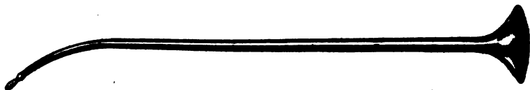
FIG. 8,633.—Ordinary mouth blow pipe.
