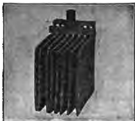
FIG. 6,315.— Battery repairs 15. Positive group showing buckled plates. A group of buckled plates which, when reassembled, will not go into the jar readily, should be replaced with a new group. Buckled plates if otherwise serviceable can be strengthened thus: Insert boards of suitable thickness between the plates and over each outside plate; place the pile in a vise, apply a gradual pressure, exercising care that the plates are not subjected to a severe strain. The condition of the negative plates is sometimes such that they may be used again with new positives. In this case the negative group should be immersed in water to prevent the plates drying out through heating or exposure to the air. If the positive plate be fairly hard, and has not lost much of its surface, it may be used again. Occasionally it happens that one or two plates in a group require replacement while the balance of the plates are in good condition. In this case new plates may be used in replacement.
