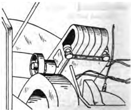
FIG. 8,036.—Method of driving a generator direct from engine fly wheel by friction pulley with spring or cushion base; the latter relieves the stress on the shaft from excessive vibration. The governor regulates the speed of the machine and prevents burning out of the lamps. The illustration shows a K-W magneto installed on an early Maxwell car.
