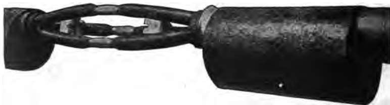
FIG. 7.413.— Cable splicing with Conducell: III. Placing in position the outer tube, lead sleeve, spaces, copper connections. The conductors are now spread apart slightly so as to make room for the porcelain spacing pieces. To avoid the possible chipping or cracking of these pieces, in bending or forming the conductors while preparing the ends, it is suggested that a forming piece made of fibre or some other such material be provided. The figure shows the lead sleeve and the outer tube of the Conducell together with the porcelain spacing pieces. The insulation on each of the conductors of both sections having been securely tied with twine, is cut entirely through to the copper strand, and the lead sleeve placed over one end of the cable, the outer Conducell sleeve over the other end. The tapered copper connections are then applied and soldered care being taken to remove all surplus solder and sharp metallic points after the connectors are soldered and the paper insulation on each conductor is then carefully tapered so as to avoid any sharp points or corners.
