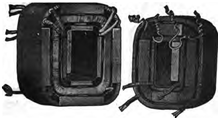
FIGS. 6,484 and 6,485.—Assembled coils of Westinghouse 10 and 15 kva. transformers; views showing ventilating ducts.
