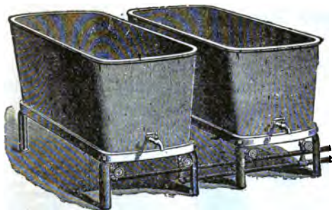
FIG. 6,364.—Heating tanks. Small shops usually depend upon gas or oil stoves placed under the various tanks or jars containing solutions that must be kept hot, such as lye, rinsing water, gold solutions, etc., as either offers a means of keeping up the desired temperature with very little trouble or expense. Larger establishments, however, find it cheaper and better in every way to use steam jacketed tanks, as here shown.
