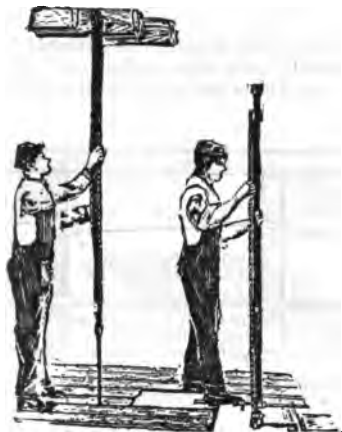
FIG. 7,114.—Boring machine for boring porcelain tube holes in knob and tube work. It will bore a hole parallel with the floor (avoiding slanting tubes) and in less time than with a brace.
