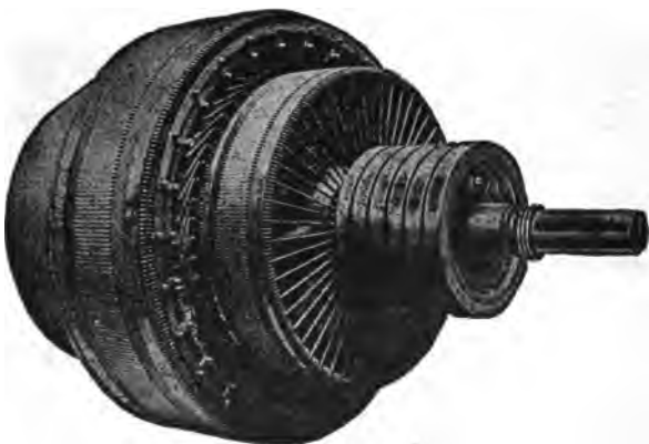
FIG. 6.612.—Armature of Westinghouse synchronous booster converter. Heavy cast yokes form the frames. They are proportioned to rigidly support the laminated steel field poles. The poles are fastened to the frame with through bolts. A lifting hook is provided on all frames.
