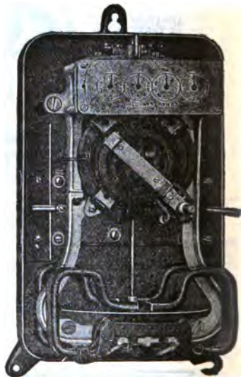
FIG. 654.—Interior view of Thompson watt hour meter (type C-6). Capacity: 5 to 600 amperes, two wire, and 5 to 300 amperes, three wire; 100 to 250 volts. The meter is supported by three lugs, the upper one of which is keyholed, and the lower right hand one slotted. This permits rapid and accurate levelling as the top screw can be inserted and the meter hung thereon approximately level.
