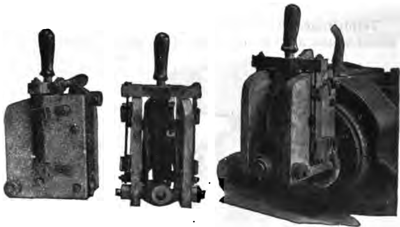
FIGS. 8,283 to 8,285.—Niles crane construction: Contact-type limit switch. It consists of a worm wheel with machined teeth actuated by a turned steel worm which is attached directly to the hoisting drum shaft. The release mechanism is operated by a positive stop on the worm wheel with a by pass attachment which prevents damage to the switch by over hoisting. The switch blades are of a quick break type operated by a powerful spring. When the switch is open the motor cannot be operated until the switch is set by hand, after which the hook can be hoisted to the maximum height in the danger zone. When the hook is out of the danger zone, the release stop is automatically reset.
