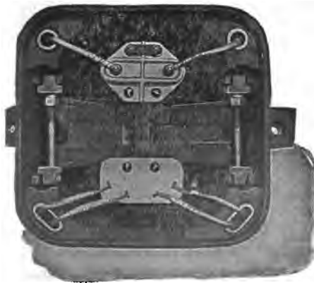
FIG. 6,490.—Top view showing core and coils in place of Westinghouse distributing transformer. The coils are wound from round wire in the smaller sizes of transformers and from strap copper in the larger sizes. Strap wound coils allow a greater current carrying conductor section than coils wound from large round wire, as there is little waste space between the different turns of the conductor. The coils are arranged concentrically with the high tension winding between the two low tension coils, the object being to improve the regulation . The low tension coils are wound in layers which extend across the whole length of the coil opening in the iron, while the high tension coils are wound in two parts and placed end to end. This construction reduces the normal voltage strains to a value which will not give trouble under any condition of service. Leads with means of preventing creeping of oil by capillary action are attached to these studs and brought out of the core through porcelain bushings.
