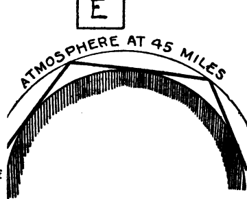
FIG. 8,458.—Reflection of electro-magnetic waves.
