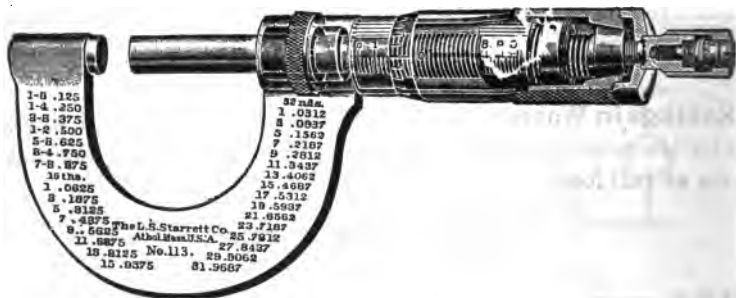
FIG. 6,916—Phantom view of Starrett micrometer calipers showing construction. Over the barrel is placed a thin graduated sleeve, which causes the base or zero line, instead of having this line marked on the barrel itself. This sleeve may be turned by means of a small spanner wrench to bring the zero line correct to compensate for wear. The thin sleeve also keeps dirt from the screw. A knurled locking nut contracting a split bushing around the spindle tightens and keeps the spindle central and true, or by a slight turn locks it firm, making a solid gauge when desired. The anvil and spindle are hardened, ground and lapped.
