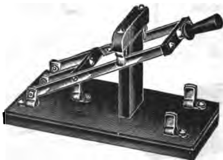
FIG. 8,479.—Aerial or antennæ switch used at Marconi stations. In operation , when thrown down, it is used for sending as it then breaks the antennæ and earth connections from the receiving tuner and completes the power circuit when the telegraph key is depressed. When thrown up, it connects the receiving tuner to the loop aerial and the ground to the G, post of the type D, tuner shown.
