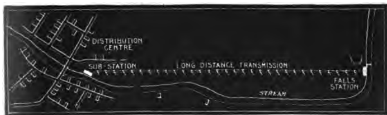
FIG. 7,889.—Example of central station located remote from the distributing center and furnishing alternating current at high pressure to a sub-station where the current is passed through step down transformers and supplied at moderate pressure to the distribution system. In some cases the sub-station contains also converters supplying direct current for battery charging, electro-plating, etc.
