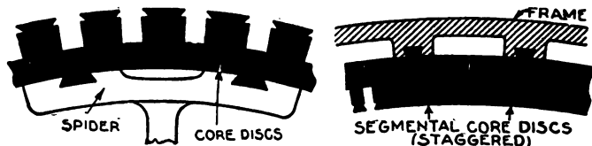
FIG. 7,715.—Large revolving armature construction with segmental discs dovetailed to spider.
