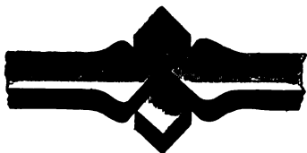
FIG. 8,651.— Glut weld. A weld in which the ends of the two parts are tapered down, and the angles filled with wedges of iron, the whole being welded together while checking the length with a trammel, excess material being subsequently cut away. This type of weld is generally used in repair work where it is necessary to maintain unchanged the length of the broken part.
