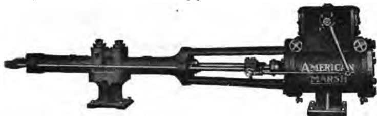
FIG. 6,188.—Hydraulic analogy of resistance. The hydraulic pump here shown with its steam cylinder of very large diameter as compared with the water cylinder is capable of pumping water against great pressure, caused by something, as a valve nearly closed, placed in the path of the flowing water which opposes its flow and thus is the cause of the pressure pumped against. Similarly, a dynamo pumps electricity through a circuit which opposes more or less its flow, this opposition being called resistance .
