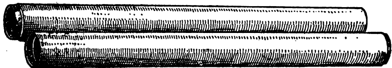
FIG. 7,354.—Fibre conduit. It consists of pipes made of wood pulp, having about the same thickness as cast iron pipe. Slip joint conduit for electrical subways is three inches inside diameter. The socket joints keep the lengths centered and make it easier to lay than a mere butt joint. It is laid in cement like iron pipe.
