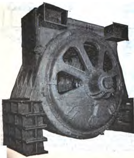
FIG. 8,220. —General Electric induction motor for merchant marine propulsion. The reliability of an induction motor on shipboard is greatly enhanced by the ease with which temporary repairs can be made in case of an electrical break down at sea, without disassembling the motor, so that the boat may continue at full or slightly reduced speed to port.
