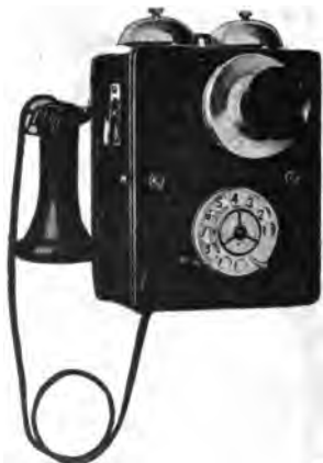
FIG. 8,420.—Automatic telephone wall type showing dial by which the subscriber makes calls without the aid of a central office operator.
