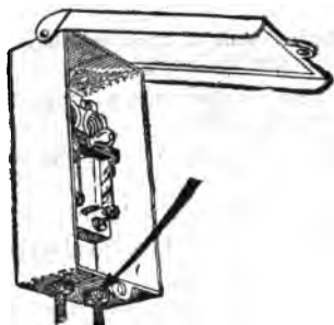
FIG. 7,258.—Method of installing switch in box; Blades are dead when switch is open; gravity closes cover of box.
