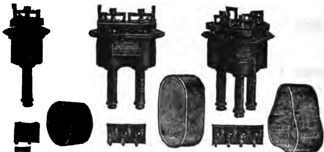
FIGS. 6,735 to 6,744. — General Electric instantaneous overload circuit opening relays, covers removed. Circuit opening relays are used chiefly in those cases where direct current for the tripping circuit is not available. Alternating current trip coils have relatively high impedance and impose a heavy volt ampere load on the current transformers. To reduce this load during normal operation the circuit opening relay is frequently used and is usually necessary where instruments and meters are to be operated on the same current transformers as the trip coils if the greatest accuracy be required. The relay contacts in the normal, closed position, short circuits the trip coil. When the relay operates on overload or other abnormal condition the contacts are opened with a quick break, sending the current through the trip coil circuit momentarily and tripping the switch. With circuit opening relays, the trip coils of the oil switch must be set to trip somewhat lower than the setting of the relay. In construction the relay consists of a solenoid with iron frame forming the support for the relay; a central plunger or armature of special construction which is picked up or released by the magnetic action of the solenoid; a plunger rod which actuates the relay contacts, which are mounted on an insulated base usually above the solenoid; a tube or plate for the calibration marking and adjustment; covers of glass or metal to keep out dust.
