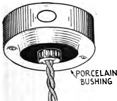
FIG. 7,262.—Drop cord fixture leaving conduct outlet box cover. A porcelain bushing must be used with all metal covers.
