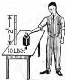
FIGS. 6,466 to 6,468.—Mechanical analogy of wattless current. If a man lift a weight any distance as from the position of fig. 6,466 to position of fig. 6,467, he does a certain amount of work on the weight giving it potential energy. When he lowers it to its original position, as in fig. 6,468, the weight loses the potential energy previously acquired, that is, it is given back to the man, the "system" (man and weight) having returned to its original condition as in fig. 6,466. During such a cycle, the work done by the man on the weight is equal to the work done by the weight on the man and no useful external work has been accomplished.
