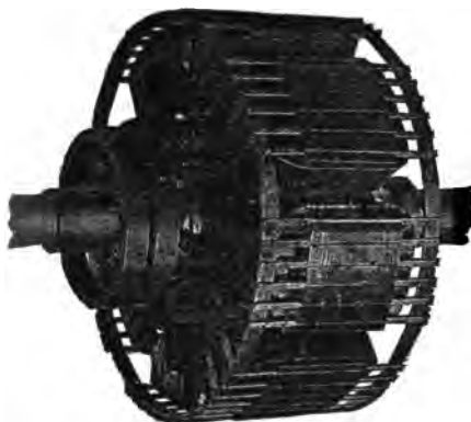
FIG. 7,699. — Westinghouse field with amortisseur or "damper" winding for 75 kva. and larger belted alternators, which prevents hunting and reduces eddy currents in the pole pieces. The copper bars of the amortisseur cage winding are arranged in partially closed slots in the pole pieces.
