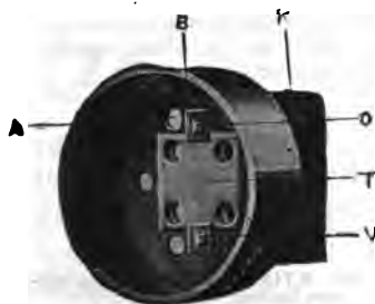
FIG. 6,733.—Notched end fuse. It consists of a strip of metal (or wire) fixed between two end pieces to fit around the terminals. This type is often proportioned so that it is only possible to place the correct size of fuse in the terminals.
