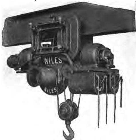
FIG. 8,286. —Niles electric mono-rail hoist, built in capacities from three-quarters to six tons. They will run on straight and curved tracks, and are generally provided with a separate motor for traversing. The hoist is self-contained in one heavy cast iron frame to which the motors are attached end on, and the power is transmitted directly from the armature shaft to the drum shaft through worm and worm wheel. The traversing mechanism is also driven by worm and worm wheel, similarly to the hoisting mechanism except that, when the trolley is arranged to run on a single I beam, a double set of transmission gears is used. The worm gear mechanism is enclosed in oil and dust proof casings, and is noiseless in operation. In addition to the braking effect obtained by use of the worm and worm wheel, a powerful electric brake is attached to the hoist motor.
