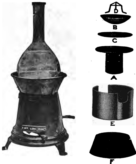
FIGS. 8,571 to 8,577. —Schaar universal electric heater with simple attachments, adapting it to the various laboratory operations for which the Bunsen burner has been used. The construction is such that the heat is concentrated at the upper and central portion of the heater, by radiation and convection, the heated air striking and surrounding the object to be heated. Crucibles and test tubes are so placed within the heater that they are heated on the sides and bottom by direct radiation. The heater coils are so arranged that any liquid spilled upon the heater falls through without injury to them. Current consumption 6.8 amperes at 110 volts on high, and 4 amperes on low. Attachment A, inserted in the heater from the top, will hold from one to four test tubes. The gauze B, is of special form for the support of round bottom flasks and evaporating dishes, and is placed in the top of the heater together with the device shown in fig. 8,571. Beakers and other flat bottom apparatus are heated in a similar manner, using the flat gauze C. The nichrome triangle D, inserted in the top of the heater, supports crucibles in position to receive the most intense heat. For reduction experiments attachment E, is placed over the heater, reduction tube allowed to rest in the slots, and the asbestos plate placed over the top. Copper oxide is thus readily reduced by hydrogen. By placing attachment F, over the flask, shown in fig. 8,571, the heat is conserved so that the time of boiling is considerably reduced.
