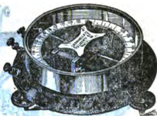
FIG. 6,684.—Bunnell horizontal galvanometer. It has two coils, one of which is of zero resistance and one of fifty ohms resistance adapting it to a variety of test.
