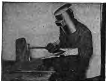
FIGS. 8,673 and 8,674.—C and C electric arc welding apparatus. Fig. 8,673, operator with one type of head shield and combination electrode holder for both metallic and graphite electrodes. Fig. 8,674, graphite electrode holder and hand shield.
