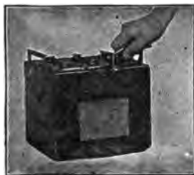
FIG. 6,307.— Battery repairs 7. Using a heated screw driver, chisel or a plumber's lead scraper dig out the compound around the edges of the covers.
