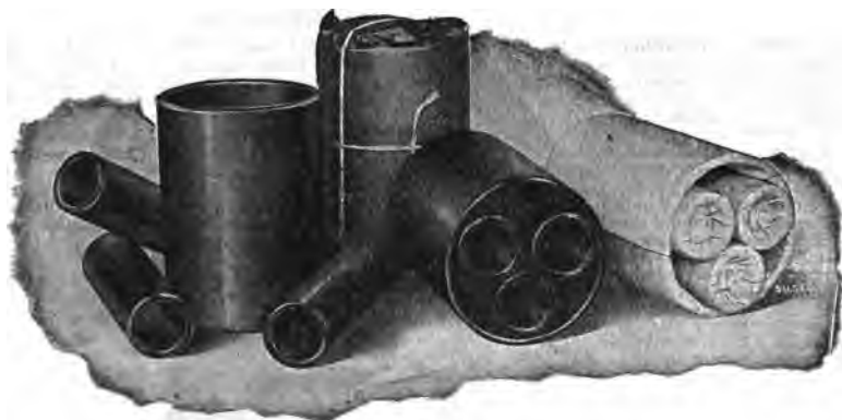
FIG. 7.397.—Standard saturated paper jointing tubes. In making , specially prepared and treated, compressed, machine laid paper is used, thoroughly saturated with an impregnating compound similar to that used in high voltage paper insulated cables, and coated on the outside with an insulating compound.
