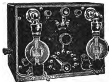
FIG. 8,497.—Professional type of audion detector. It is provided with two super-sensitive audion bulbs, high voltage local battery, potentiometer switch graduated to show voltage at any point, switch to change from one bulb to the other, and rheostat to change brilliancy of filament. This detector is used by the U. S. Army and Navy, and is furnished in oak and hard rubber; size, 9\frac{1}{4} by 9 by 7 inches. Three dry cells to light filament are necessary.
