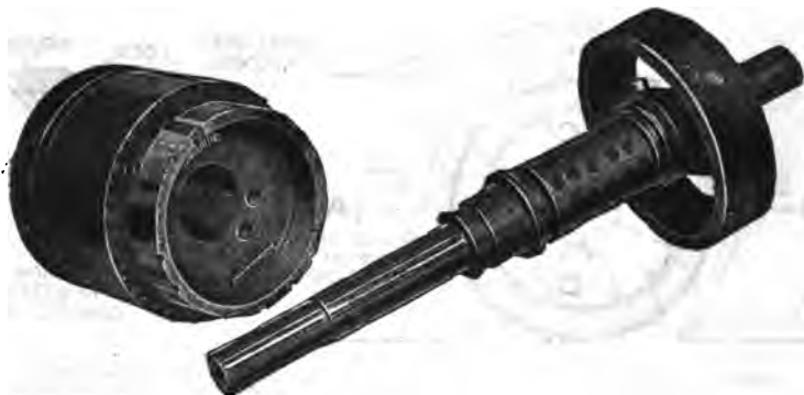
FIGS. 7,816 and 7,817. —General Electric dissembled clutch as used on clutch type, single phase (KS) induction motor. In starting , the armature revolves freely on the shaft until approximately 75 per cent. of normal rated speed is reached. The load is then picked up by the automatic action of a centrifugal clutch, which rigidly engages an outer shell, keyed directly to the shaft. The brass friction band of the clutch is permanently keyed to the pulley end of the armature.
