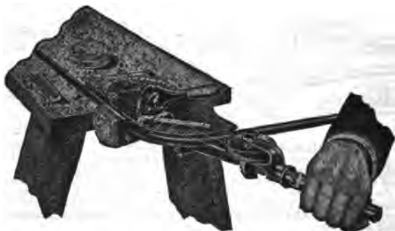
FIG. 7,147.—Machine for making quarter bends. This type of a tool should be used on large jobs where a number of bends the same size is desired.
