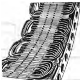
FIGS. 7,755 to 7,757.—Separate coils, and section of Allis-Chalmers alternator with coils in place.
