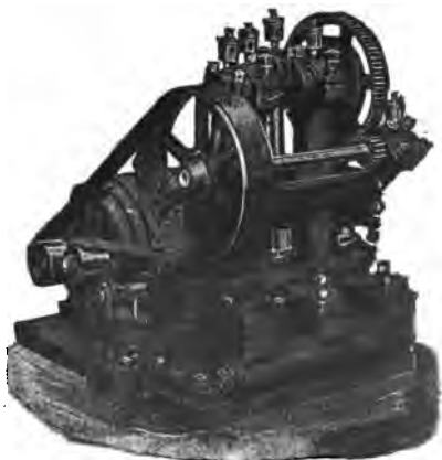
FIG. 8,243.—Deming single acting plunger triplex pump with double reduction combination short belt and spur gear drive . This type has the desirable features of quiet running and compactness. When a rawhide pinion is used practically all noise is eliminated.
