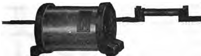
FIG. 6,764.—General Electric magnetic blow out arrester for line use. It consists essentially of a small spark gap which is in series with a resistance and between the poles of a magnet. The spark gap and the magnet are mounted within porcelain blocks in such a way that the discharge arc is blown by the magnet through an arc chute and a cooling grid which is also held by the porcelain.
