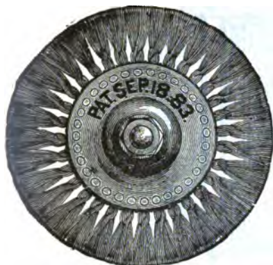
FIGS. 6,379 and 6,380.—Hanson and Van Winkle swing type, circular steel wire, casting brush. The steel wires are twisted in knots and the knots are hung on rods around the hub, as shown in fig. 6,379, so that they will turn around the rods if the work be held too close to the brush wheel. In using the brush the work should be held so as to be just in contact with the ends of the wires. The brush shown is about 15 inches in diameter, and should not be run much faster than 1,000 r.p.m.
