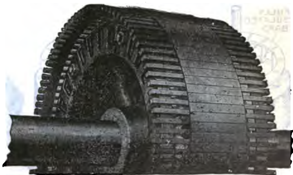
FIG. 7.795.—General Electric welded form of end ring construction on squirrel cage armatures. Space limitations make it difficult to provide parallel soldered rings of sufficient area for large motors; hence, on such machines welding is resorted to, as shown. The ring in welded construction is placed beneath the bars at each end of the armature. Short radial bars are welded to the edges of these rings and to the inductors or squirrel cage bars, thereby making good electrical contact.
