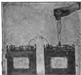
FIG. 6,345.— Battery repairs 45. In burning connectors and terminals to the posts, melt the top of the post, then the edges of the hole in the connector. Melt strips of antimonious lead and allow the molten metal to run into the hole in the connector. Care must be taken to see that the top of post and inside edges of the connector are melted together before applying additional lead. If this be not done, the connection will surely pull loose. Care should also be taken not to melt the outer edges of the connector. Practice will be found necessary.
