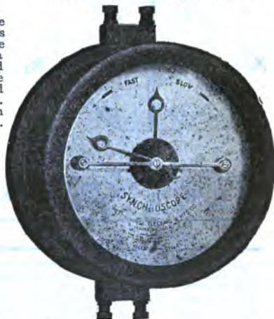
FIG. 6,810.—Westinghouse rotary type of synchroscope or synchronism indicator. The indication is by means of a pointer which assumes at every instant a position corresponding to the phase angle between the pressures of the bus bars and the incoming machine, and therefore rotates when the incoming machine is not in synchronism. The direction of rotation indicates whether the machine be fast or slow, and the speed of rotation depends on the difference in frequency. The pointer is continuously visible, during both the dark and light periods of the synchronizing lamps.
