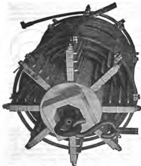
FIGS. 6,735 to 6,744. — General Electric instantaneous overload circuit opening relays, covers removed. Circuit opening relays are used chiefly in those cases where direct current for the tripping circuit is not available. Alternating current trip coils have relatively high impedance and impose a heavy volt ampere load on the current transformers. To reduce this load during normal operation the circuit opening relay is frequently used and is usually necessary where instruments and meters are to be operated on the same current transformers as the trip coils if the greatest accuracy be required. The relay contacts in the normal, closed position, short circuits the trip coil. When the relay operates on overload or other abnormal condition the contacts are opened with a quick break, sending the current through the trip coil circuit momentarily and tripping the switch. With circuit opening relays, the trip coils of the oil switch must be set to trip somewhat lower than the setting of the relay. In construction the relay consists of a solenoid with iron frame forming the support for the relay; a central plunger or armature of special construction which is picked up or released by the magnetic action of the solenoid; a plunger rod which actuates the relay contacts, which are mounted on an insulated base usually above the solenoid; a tube or plate for the calibration marking and adjustment; covers of glass or metal to keep out dust.
