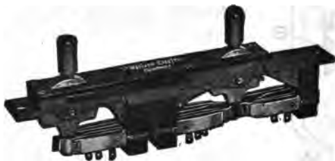
FIG. 8,391.—Modern ringing keys. In order to meet the needs of every calling subscriber, the operator must perform several different acts in shifting and changing circuits and to facilitate this work, devices to simplify it as much as possible have been developed. The modern ringing keys have greatly helped in the saving of the operators' time. By throwing the little levers a hard rubber bushing makes or breaks the contacts at the springs and throws alternating current ringing power into the line. When the finger pressure is released, the levers fly back again into normal position.
