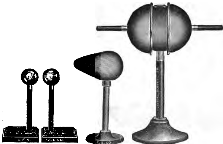
FIGS. 6,119 to 6,121.—Electrostatic apparatus. Fig. 6,119 induction spheres so mounted on insulating support that they can be brought into contact. Useful in connection, with fig. 6,118 for showing the separation of positive and negative electricity by induction. Fig. 6,120, ellipsoidal conductor for showing unequal distribution. Fig. 6,121 Biot's hemispheres with pair of their nickel plated brass hemispheres with rubber handles. Charge on outside of globe may be removed by placing hemispheres in position shown.
