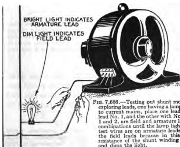
FIG. 7,685.—Interpole motor. The object of the interpole winding is to assist in the reversal of the current under the lamp lights. If it burns brightly, test wires are on armature leads; if dimly, they are on the field leads because in this case the considerable resistance of the shunt winding cuts down the current and dims the light.
