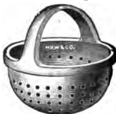
FIGS. 6,372 and 6,373.—Various dipping vessels. Fig. 6,372, deep glazed earthenware dipping basket; fig. 6,373, shallow glazed earthenware dipping basket. The aluminum basket is adapted for use in washing and dipping in all acid solutions, but cannot be used in potash solutions. Different shapes and sizes of basket are required for various kinds of work. Successful dipping depends, however, chiefly upon quick and careful handling rather than upon the shapes of the dip, therefore, the holes in these baskets should be as large as possible, so as to allow the acid or cyanide solution to drain out quickly.
