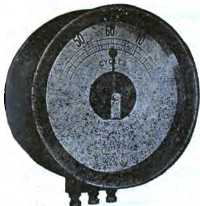
FIG. 6,809.—Westinghouse induction type frequency meter. The normal frequency is usually at the top of the scale to facilitate reading. The damping disc moves in a magnetic field, thus damping by the method of eddy currents. The standard meters are designed for circuits of 100 volts nominal and can be used for voltages up to 125 volts. For higher voltages, transformers with nominal 100 volt secondary should be used.
