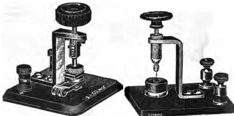
FIG. 8,488.—Peroxide of lead detector. A flat piece of peroxide of lead is clamped between a platinum surface and a flat piece of lead. Binding posts connect to these two electrodes and are marked + and —. The positive pole of a battery is connected to the platinum electrode at the binding post marked +.
