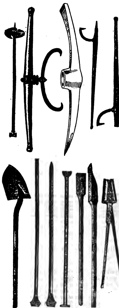
FIGS. 7,295 TO 7,306.—Pole construction tools. Fig. 7,295, long handled digging shovel; fig. 7,296, digging bar, fig. 7,297, crow and digging bar; fig. 7,298, tamping and digging bar; fig. 7,299, wood handle post hole auger; fig. 7,300, slick digging tool; fig. 7,301, post hole auger; fig. 7,302, carrying hook; fig. 7,303, tamping bar; fig. 7,304, split wooden handle post hole auger; fig. 7,305, cant hook; fig. 7,306, socket peavey.
