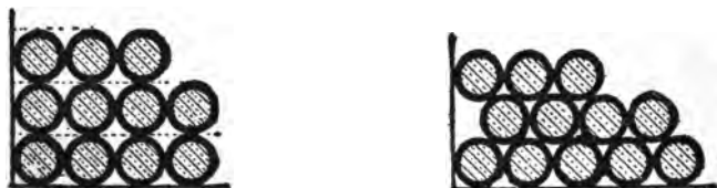
FIGS. 7,566 and 7,567.—Square and hexagonal order of "bedding." The term bedding is an expression used to indicate the relation between the cross sectional area of the winding when wound square, as in fig. 7,566, and when wound in some other way, as in fig. 7,567. In the square order of bedding, the degree of bedding equals zero.
