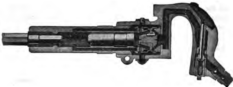
FIG. 7,965.—Thor short stroke pneumatic hammer for chipping, caulking and tube beading, etc. A feature is the valve mechanism. The valve block consists of two solid cylindrical parts. The exhaust passes below and above the valve.
