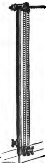
Figs. 7,294 and 7,295.—Henderson's boring machine fig. 7,294, extended; fig. 7,295, telescoped. This machine is for boring holes through joists from the floor. It has ball bearings and universal bit holder and is built to telescope to 4\frac{1}{2} feet and extend 2 feet.
