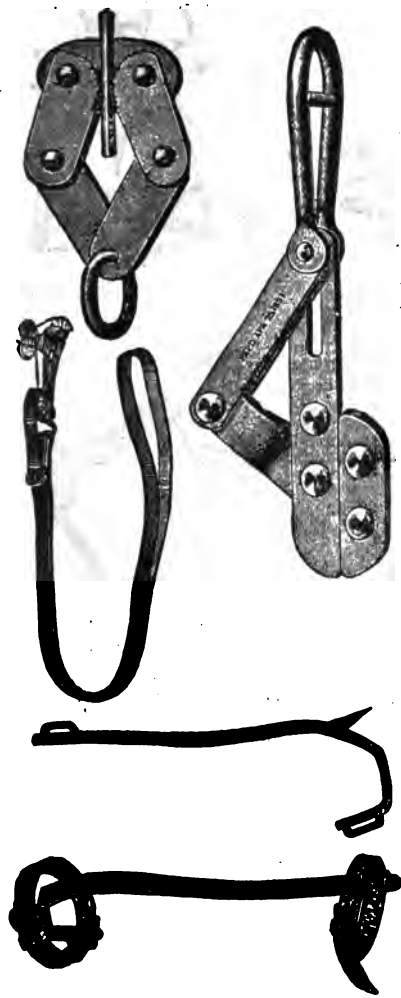
FIGS. 7,318 to 7,322.—Lineman's tools. Figs. 7,318 and 7,319, Eastern pole climbers, with and without strap, or attaching to legs; fig. 7,320, portable vise with strap for pulling up the slack in splicing; figs. 7,321, one form of "come along." The wire is inserted between jaws and is held fast when tension is applied to the ring; fig. 7,322, an improved form of "come along" or wire stretcher. The jaws which grip the wire are smooth and remain parallel in closing, thus the wire is not scratched or indented, as with circular jaws having teeth.
