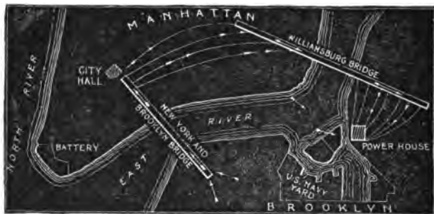
FIG. 6,350.—Electrolysis in lower New York. The figure illustrates current movements as discovered. The power house is located near the navy yard in Brooklyn. A portion of the returning currents, as shown by arrows, flows over the New York and Brooklyn bridge to Manhattan, thence north to Williamsburg bridge via underground mains, subway structures, and other metals, and passes over that bridge back to Brooklyn, thence through mains to rails and negatives, to power house. In this case damage may be expected at three points: 1, where currents leave bridge metals on the Manhattan side; 2, where they leave pipes to enter Williamsburg bridge; 3, where they leave same bridge for pipes in Brooklyn side. When the two bridge structures are connected in Manhattan as proposed, then there will be further changes in the direction of current. Before the Williamsburg bridge was built, these currents recrossed through the river bed, leaving mains all along the docks in the Manhattan side, for the river, and leaving the river for mains or other metals along the docks of the Brooklyn side. Traces of these currents have been found as far north as 23rd St., a distance of over two miles from the Brooklyn bridge. Since the Williamsburg bridge has been built, nearly all traces of these currents flowing north of it have disappeared, showing that the mass of metal composing the structure acts as a short circuit or path of lower resistance which carries practically all of the returning currents flowing from Manhattan back to Brooklyn.
