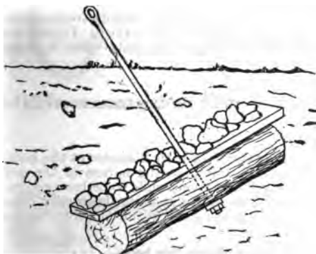
FIG. 7,315.—Guy anchor log in position.
