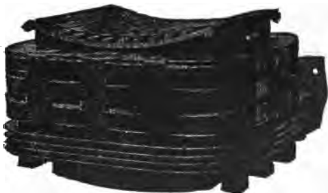
FIG. 6,592.—Westinghouse pole construction for converters. The poles are built of up sheet steel laminations held together with rivets. Projections in the inner ends of the poles form seats for the field coils and hold them in position. Copper dampers set in slots in the pole faces insure stable operation. Rotary converters for railway service are almost invariably compound wound. The series windings are formed of bare copper strap. The shunt windings are of insulated copper strap or wire. Spaces between coil turns and sections are provided for ventilation.
