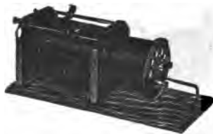
FIG. 8,483.—Loose couple receiving transformer with variable contacts.
