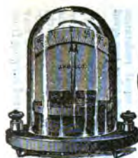
FIG. 6,683.—Breguet upright galvanometer with glass shade.
