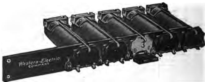
FIG. 8,392.—Mounted trunk drops. Tubular trunk drops are mounted on a metal strip each being held by two small screws underneath the drop shutter. The tubular casing of each drop is soft iron inside of which is the drop winding, the ends of the coil wires terminating at lugs which protrude from the casing and are insulated therefrom. The drop shutters are then screwed fast to the metal strip and adjusted so that they may fall easily when the armature is held up by the magnet.
