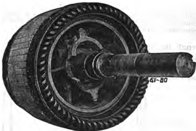
FIG. 7,810.—View of armature interior of Wagner polyphase induction motor with wound armature, showing the centrifugal device which at the proper speed short circuits all the coils, transforming the motor to the squirrel cage type. The winding is connected with a vertical "commutator" so called. Inside the armature are two governor weights, which are thrown outward by the centrifugal force when the machine reaches the proper speed thus pushing a solid copper ring (which encircles the shaft) into contact with the inner ends of the "commutator" bars, in this way completely short circuiting the armature winding.
