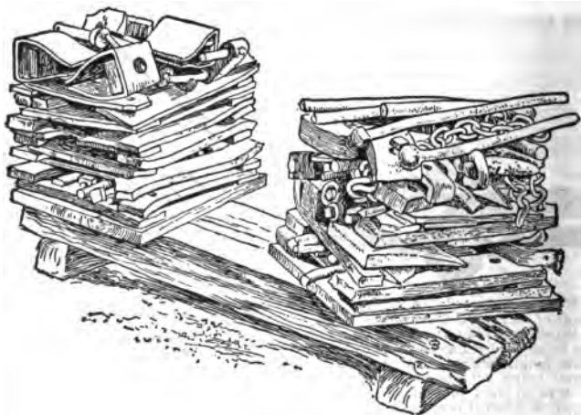
FIG. 8,653.— Fagoting. The pile is started with a flat piece of iron, generally fagoted up of small pieces and the pieces of scrap iron piled on top of this, making a firm rectangular pile with large pieces around the outside and small pieces in the center, or the flat piece on the board may be omitted. It is then heated in a furnace and welded under a steam or a machine hammer.
