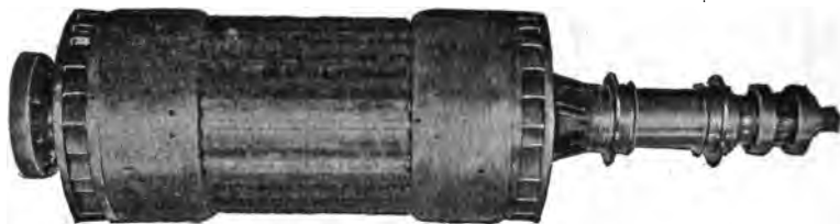
FIG. 8 218.—General Electric revolving field of alternator of the turbine driven unit shown in fig. 8,223.
