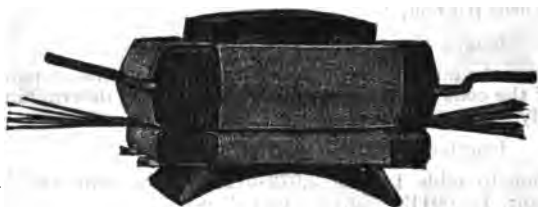
FIG. 7.832.—Fairbanks Morse field coils of type TR machine. In construction, the coils are wound upon iron forms, each layer treated with insulating compound. Afterward they are removed from the forms and baked hard and dry and finally wrapped with insulating materials and finished with black insulating enamel.
