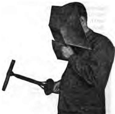
FIGS. 8,673 and 8,674.—C and C electric arc welding apparatus. Fig. 8,673, operator with one type of head shield and combination electrode holder for both metallic and graphite electrodes. Fig. 8,674, graphite electrode holder and hand shield.
