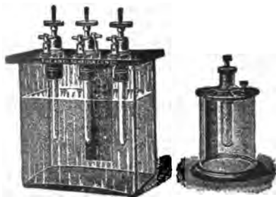
FIGS. 8,708 and 8,709.—Wehnelt electrolytic interrupters. Fig. 4,617, 3 point interrupter; fig. 4,618, 1 point interrupter. In the multi-point type two or more anodes can be used at one time in parallel, thus more current can be passed through the primary.
