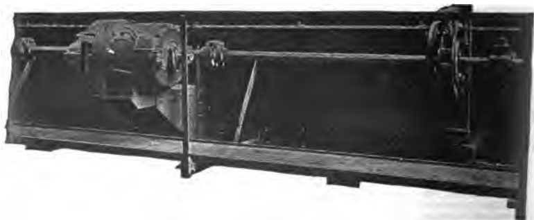
FIG. 8,279.—Niles crane construction: Bridge drive for box section girders. The web plates of the box section girders are reinforced by heavy stiffening angles, placed near the bridge drive motor and are connected by diaphragms, preventing distortion of the girders by motor or gears. A substantial platform with angle iron hand rail extends along the girder on the bridge drive side, providing easy access to the bridge motor, gears and bearings.
