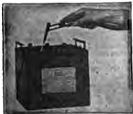
FIG. 6,308.— Battery repairs 8. Again using a flame, heat the top of the covers to soften the underlying compound. Insert a screw driver under the covers and pry them off gently. Do not attempt to force them off but use more heat until they lift easily.
